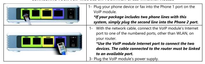
The VoIP module only works with phone devices (fax or telephone). NEVER use a cable to connect the Phone 1 or Phone 2 ports to a wall phone outlet. This could damage your conventional phone line.
